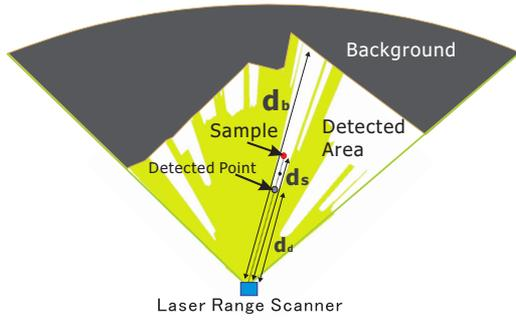
Fig. 4. Parameters for observation model of laser range scanner
