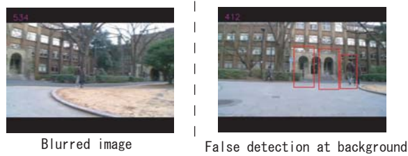
Fig. 7. An Example of mistake due to blurred image and cluttered background
