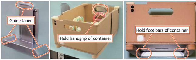
Fig. 7. Snapshot of wall hanger for i-Container.
