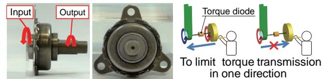
Fig. 14. Snapshot and function sketch of torque diode.
