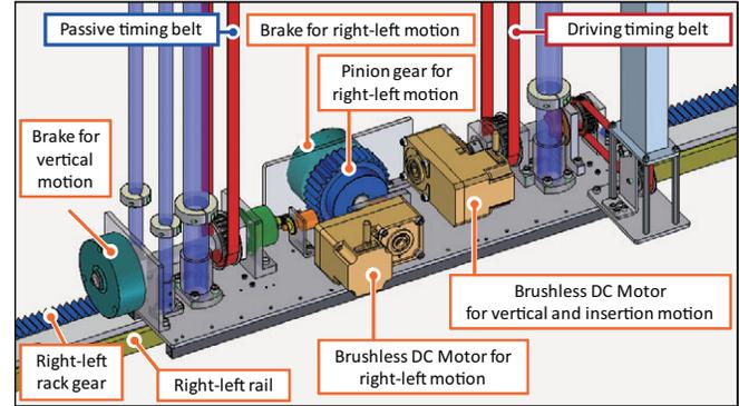
Fig. 13. Brushless DC motors and rack-and-pinion at the bottom plate.
