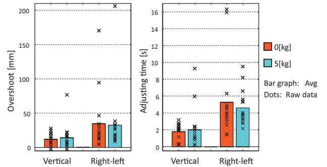
Fig. 20. Averages and distributions of the overshoot and the adjusting time in manual operation.
