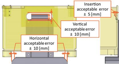
Fig. 8. Error tolerance capability of wall hanger.
