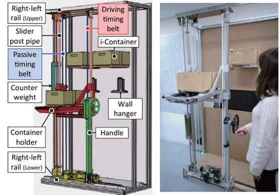
Fig. 5. Overview and snapshot of non-industrial stacker crane.
