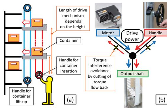
Fig. 3. (a) Restriction of drive mechanism for manual operation (b) Cutting off of torque flow back.
