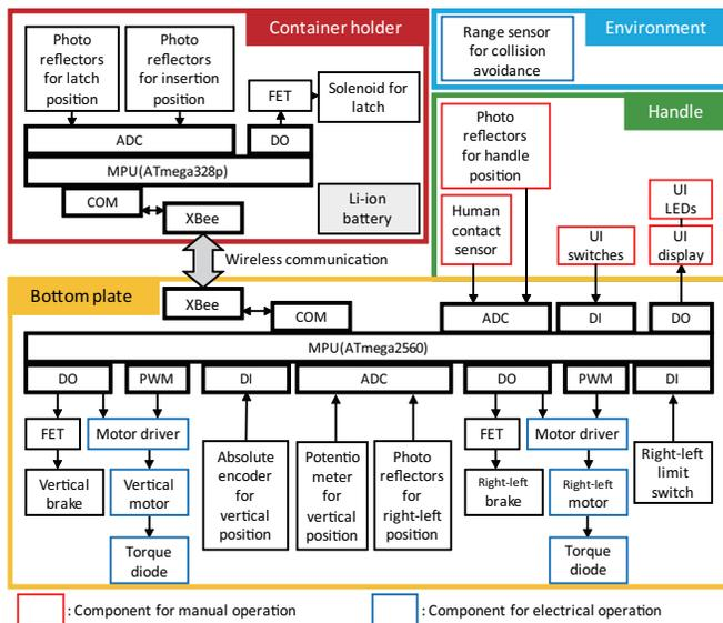
Fig. 12. Block diagram of expansive components for electrical driving.
