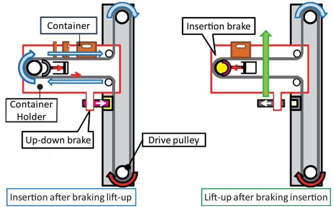
Fig. 9. Sketch diagram of the 2 DOF sharing mechanism.
