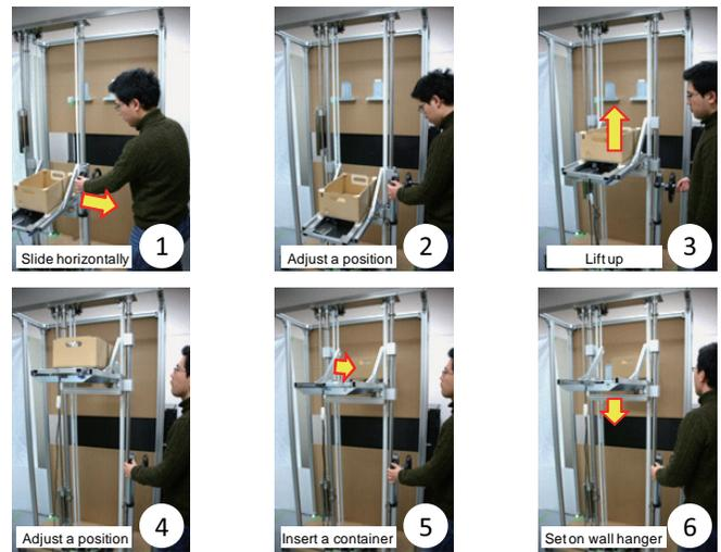
Fig. 6. Sequential snapshots of container storage motion.
