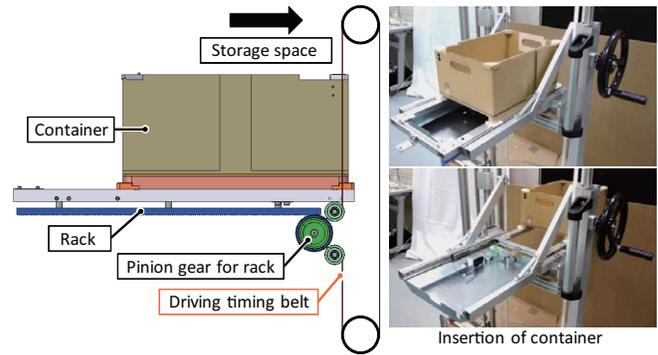
Fig. 10. Snapshot of the implemented 2 DOF sharing mechanism.
