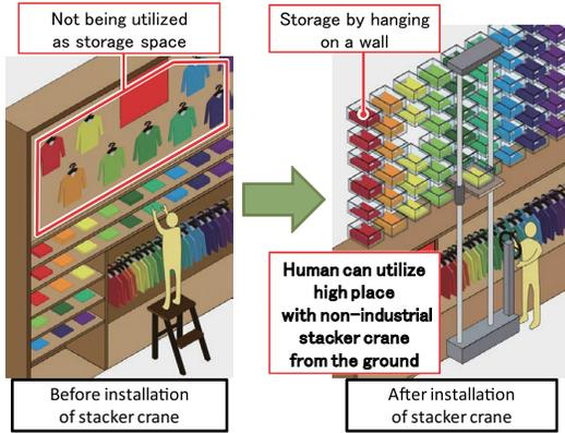
Fig. 4. Conceptual sketch of the non-industrial stacker crane.
