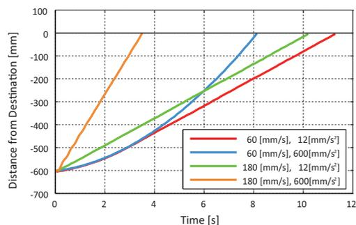
Fig. 16. Measured data examples of lifting up motion in electrical driving.
