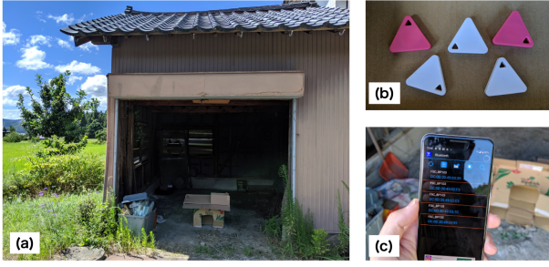
Fig. 5: Laboratory environment: (a) scenery of the experiment's location; (b) beacons representing a crowd carrying smartphones; (c) there were no BLE devices other than the tested ones.
