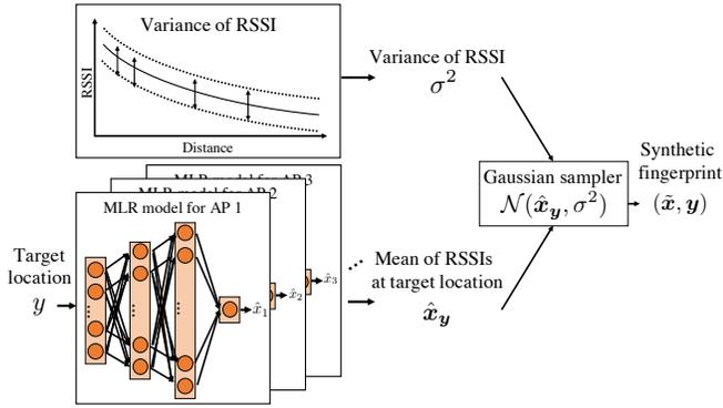
Fig. 5: Synthetic fingerprint generation with MLR and Gaussian sampler
