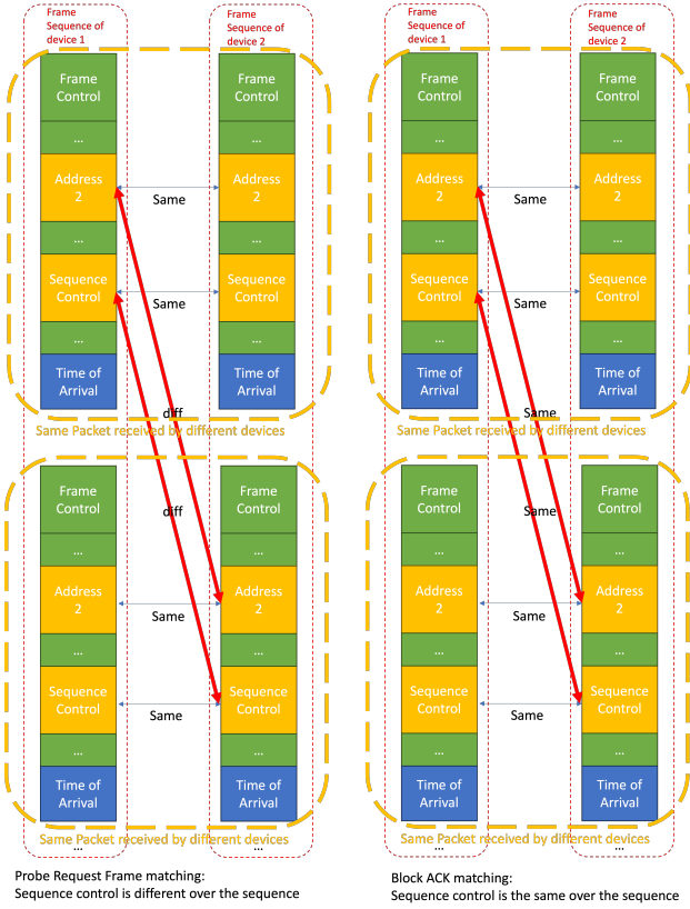
Fig. 2 Properties in frame information for frame matching of Probe Request Frame and Block ACK Frame
